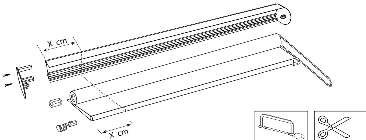
Disassemble the roller blind at first. Then shorten the upper rail, the fabric, the cloth windind shaft and the wheighting rail to your desired lengt (see picture - lengt X). Reassemble the roller blind. At assembly, make sure that all extracted parts are placed in their predetermined place.
