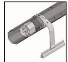
4. Run the roller shutter up until it almost reaches the desired end point. (If the motor stops already automatically, continue from point 5). The roller shutter locking bar should still be visible from the outside. Now turn the upper setting pin in the minus direction until the motor reaches the upper setting point in good time. Now position the switch upwards and carry out the fine setting process. For this, your turn in the plus direction until it reaches the desired cut off point.
